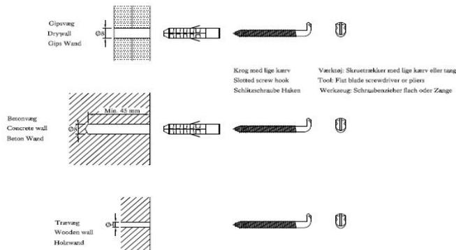
Template for drilling for mounting screws.
